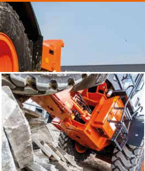
The optional belly guard provides added protection.
