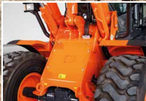
The front frame of the ZW150-6 has been reinforced.
