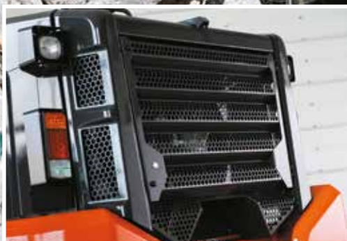
New rear grill protects radiator compartment.
